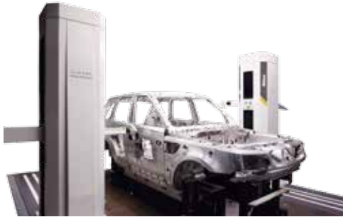
LK H-R premium series twin-rail mounted horizontal arm CMM with walk-on covers
